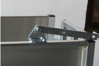
Attach the lever to the outside of the mounting bracket. The short part of the lever must face inward. The rounded head screw must point from inside to outside.
