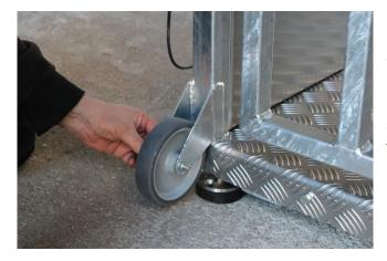
Mount the two wheels at the front of the scale. One disc each is to be installed between the wheel and the fastening latch. The wheels have a mounted inner socket, and the screws can therefore be tightened.
