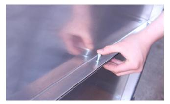
Mount the 4 screws per side to attach the lower side panels to the upper ones.
