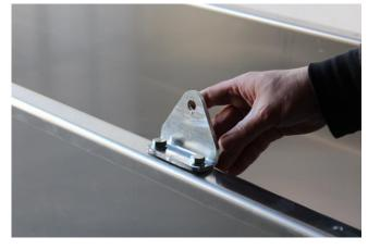
Attach the mounting bracket on the lefthand side of the scale with two M8 screws. The standing component must point inward.
