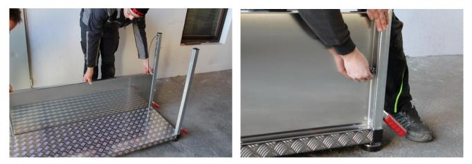
The upper two side panels are different. The left side panel has three holes on top, the right side two holes. Place the upper side panels also with the smooth surface facing inwards, while paying attention to the cables. Secure the panels with two screws each at the front and back, too. Don't tighten the screws yet.
