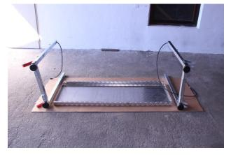
Lay the frame part with the wheel fastenings sideways on a flat surface. Be careful not to damage the attached cables.
